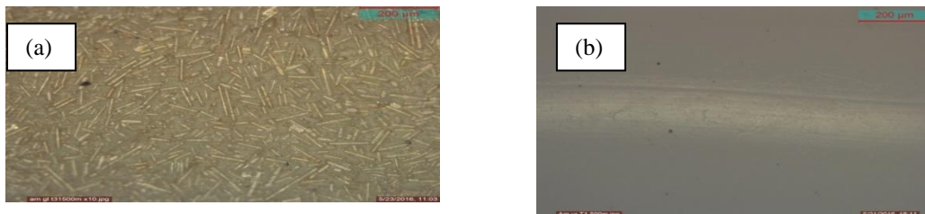
Figure 7. Optical microscope image after the sliding distance of 2000 m at 20 N load of (a) 25% glass filled and (b) virgin PTFE.
